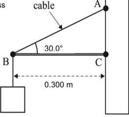
(b) Calculate the reaction force the hinge exerts on the beam at Point C.
